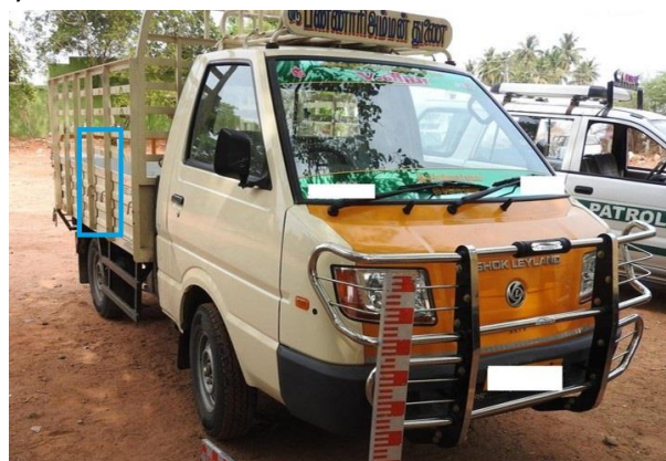
Fig. 1. Example to show the alterations/ extra fitment protrusions on cargo bay
